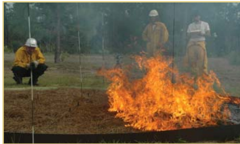
Center researchers test burn mulch to determine the safest for use around homes.
