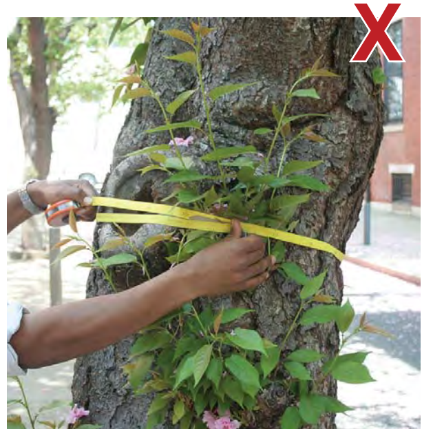
Example of measuring DBH INCORRECTLY d-Tape should go under any sprouting and also avoid any irregularities.
