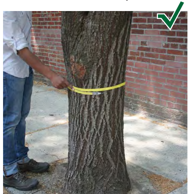
Example of measuring DBH CORRECTLY d-Tape height adjusted to avoid trunk cavity and irregularity
