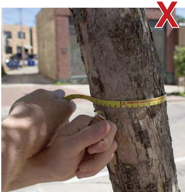
Example of measuring DBH INCORRECTLY d-Tape is too loose and should be perpendicular to trunk
