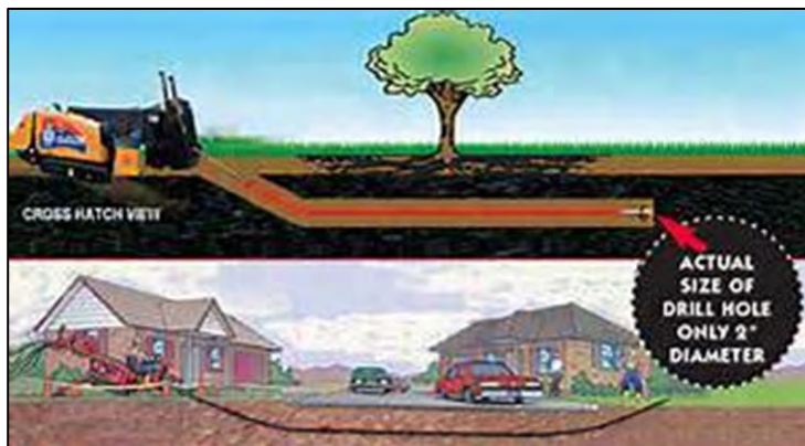
Directional Boring Machine
