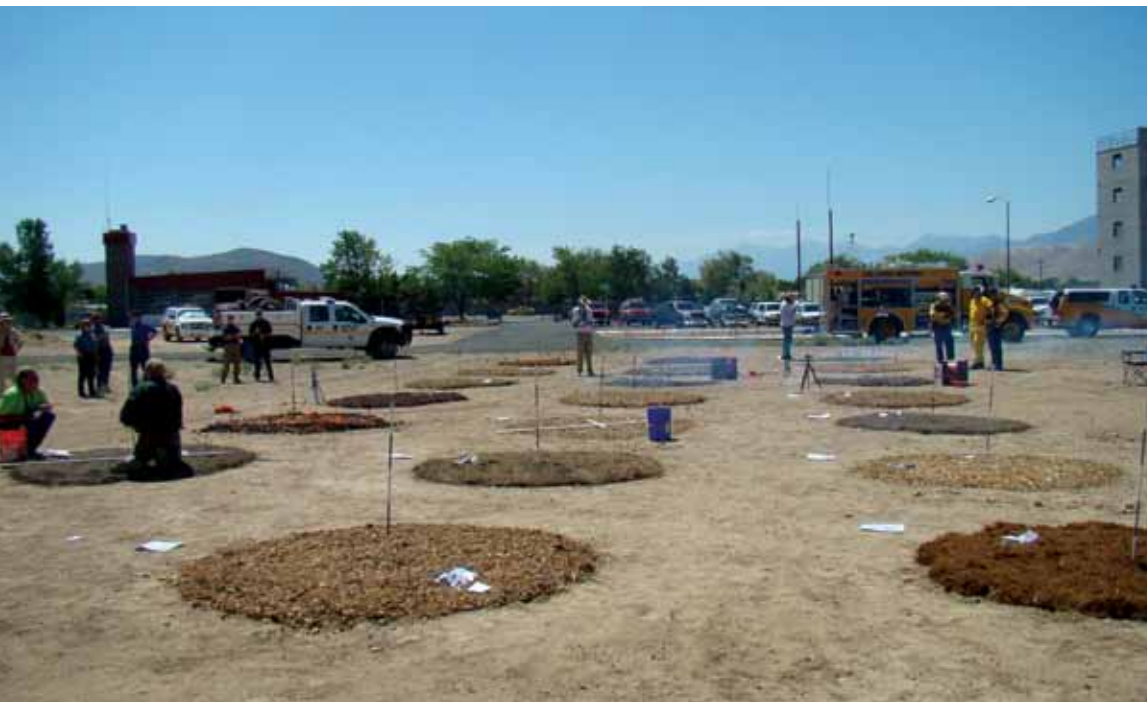
◀ Figure 2. The eight different mulch treatments were replicated three times and randomly positioned within the plot layout on May 28, 2008. After being exposed to the elements for over 2½ months, they were ignited on Aug. 14, 2008.
