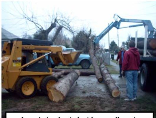
Logs being loaded with a small truck mounted hoist for transport to the sawmill
