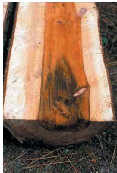
Figure 3.10 - 3.11. Rotten or punky wood or cavities indicate advanced decay.
