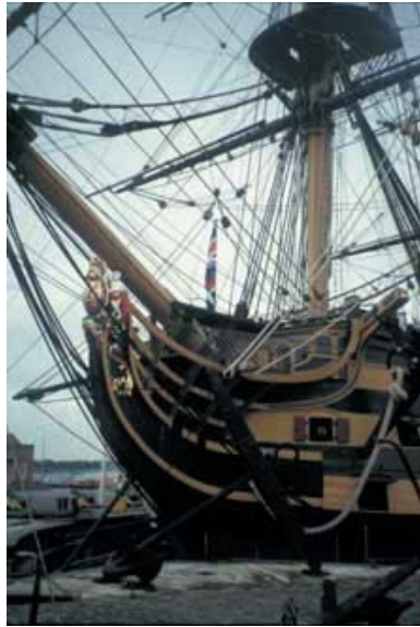
Figure 5.10. H.M.S. Victory, the flag ship of Vice-Admiral Lord Nelson at the Battle of Trafalgar, illustrating the use of flexible and rigid braces between masts and spars.
