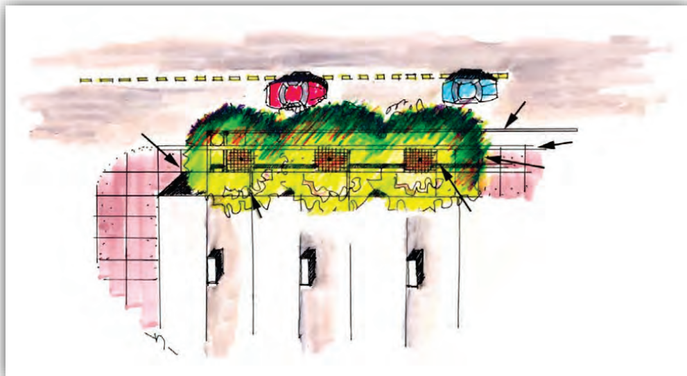
Figure 3. Plan view of linear stormwater tree pit. ( Watershed Forestry Resource Guide , Center for Watershed Protection and USFS Northeastern Area)
