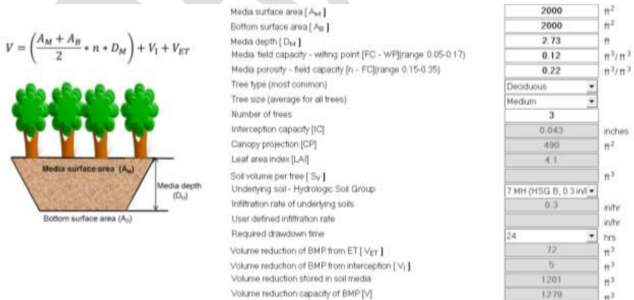
Figure 5 —A MIDS Calculator Tree Trench BMP input screens showing tree/soil inputs (white boxes) and model outputs (gray).
