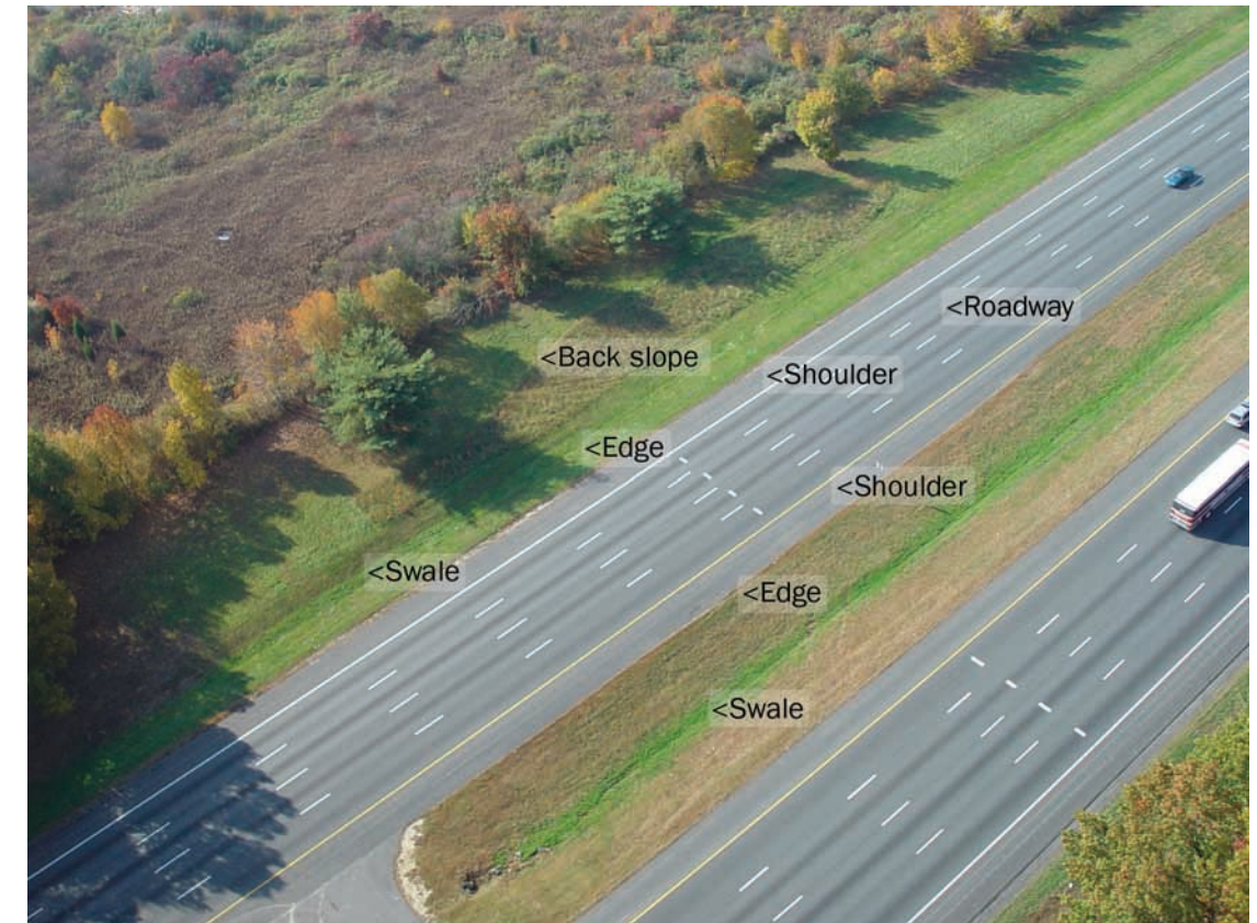
Typical zones on a dual highway.
