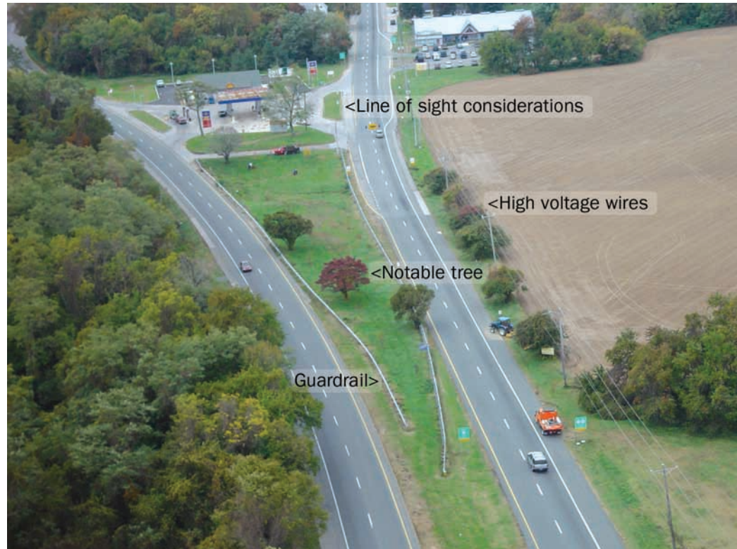
Vegetation planning for this site must document roadway limitations and existing elements such as high voltage wires, line of sight considerations, guardrails and existing trees; using the Roadway Limitations Checklist.
