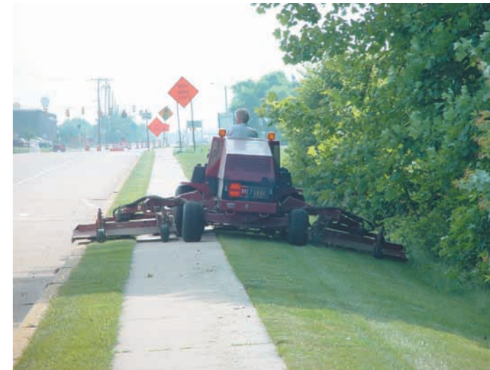
Routine mowing is expensive. However, on a limited basis, especially on relatively even surfaces, it is an effective maintenance strategy resulting in an attractive appearance with a high degree of utility. Along Wyoming Road in downtown Newark, mowed cool-season turf is a neat and practical groundcover for the relatively small area between curb and sidewalk, and between sidewalk and woods edge.
