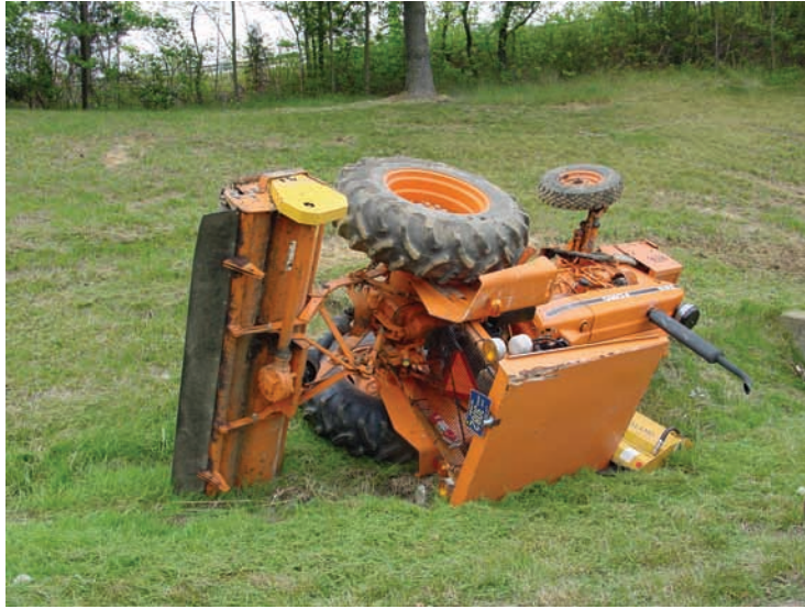
Though no one was injured in this mishap, the long-term safety solution is to adjust design and management strategies to reduce mowing on slopes and drainage swales.
