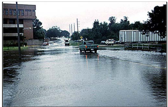
Figure 22. In the urban landscape, impervious surfaces produce more runoff in a shorter period of time.
