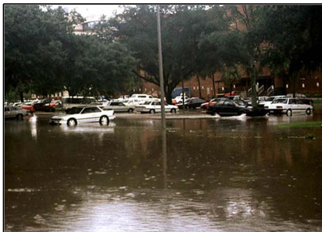
Figure 29. Reduced storage, high runoff rates, and concentrated peak flows will often result in flooding in urban landscapes.
