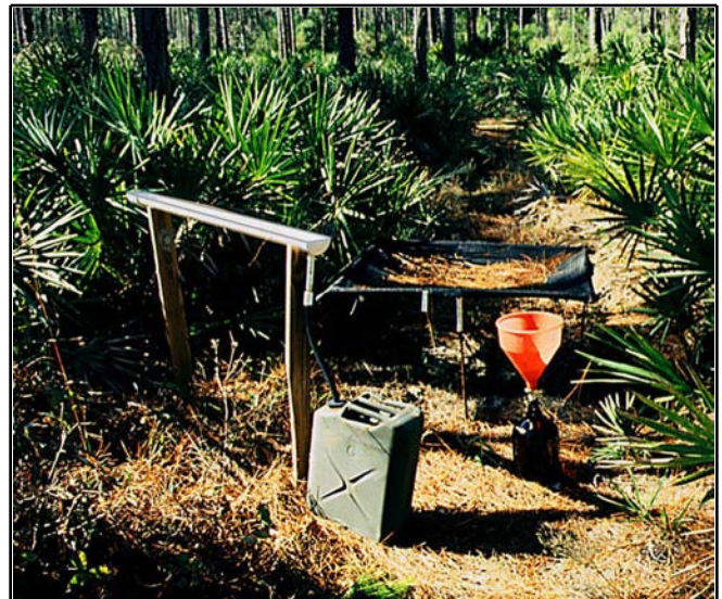
Figure 5. Through-fall is measured with troughs and funnels placed under the canopy. The measurements are often correlated with canopy leaf area, which is estimated in this figure with leaf fall traps.
