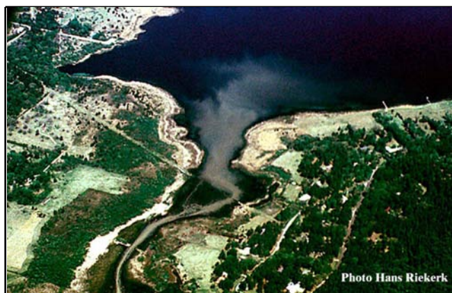
Figure 32. Pollution washed from altered landscapes is referred to as non-point source pollution. This aerial photo shows a sediment plume in a lake washed from upstream construction in an urban watershed. Photo by Hans Riekerk.
