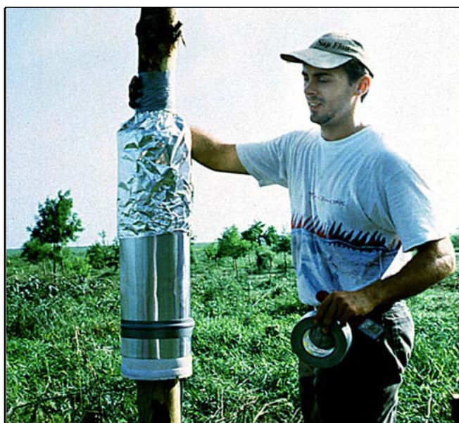
Figure 8. A sap flow gage measures sap flowing up the tree trunk on its way to be transpired from the leaves.
