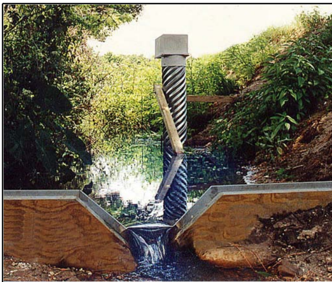
Figure 37. Weirs also measure flow, and they are less expensive than flumes. However, they dam up the water behind them which can cause many problems.
