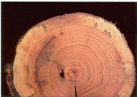
Figure 4.--Dull, yellow sapwood decay with black zone lines
