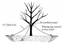
Trees less than 2 inches in caliper will not need to be staked unless the location is very windy. Stake larger trees according to the illustration.
