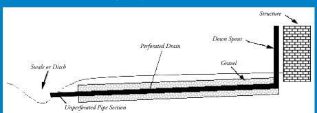
If the site does not allow for regrading or installing diversions; or if surface depressions, a high water table, or hydric soils are present; an underground drainage pipe may be necessary. Pipe grades should be gentle enough to allow water to enter but provide enough fall to drain readily. The water should empty into an existing drainage ditch or curb inlet where possible.
