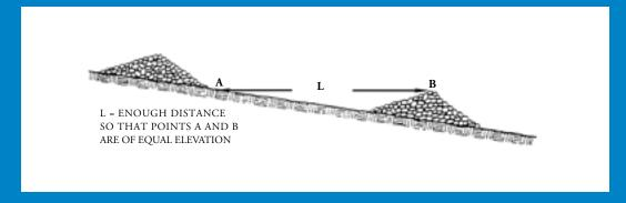
To stop concentrated flows on slopes that drain 5 acres or less, install a series of rock check dams. Place graded, size 2- to 10-inch stone the entire width of a ditch or drainageway so that the center is lower than the edges. (See middle diagram.) Stone piles should not exceed 24 inches in height. A series of check dams should be spaced apart so that the toe of the uphill dam is at the same elevation as the top of the downhill dam. Do not install check dams in streams.
