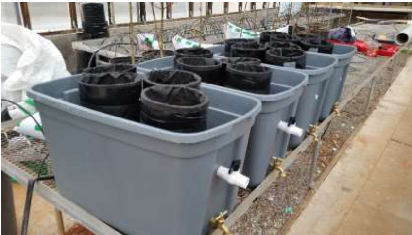
Large, plastic tubs were fitted with 1/2" PVC ball valves and brass gate valves to help control water volume within the system. The ball valves act as the under-drain and the gate valve functions as the belowground infiltration of the soil surrounding the system.
