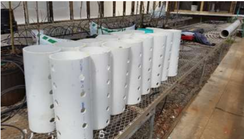
Schedule 40 PVC pipes were cut to 15" lengths and 1" diameter holes were bored along four sides at 3" intervals. Holes bored along the north/south walls began at 3" from the top edge. Holes bored along the east/west walls began at 1.5" from the top edge.
