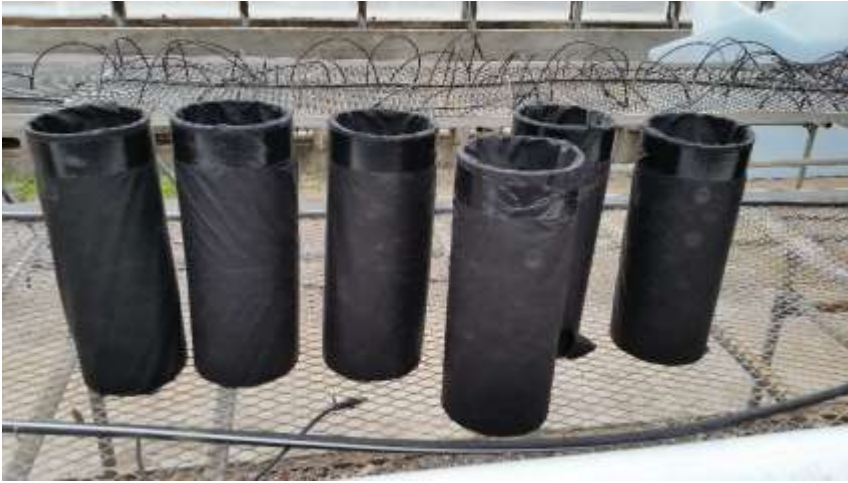
Each section was wrapped in black, woven, synthetic landscape fabric to help prevent migration of potting soil within the pots to the gravel profile during watering.
