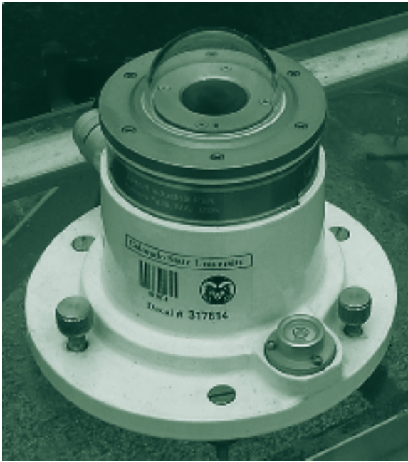
Figure 5. Scientists use special sensor equipment placed under a tree or on the ground to measure the amount of the sun’s radiation reaching the ground. Notice the clear bubble on the top of the equipment.
