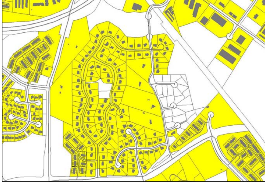
Figure 1. Use GIS to select out developed parcels (parcels with buildings on them)
