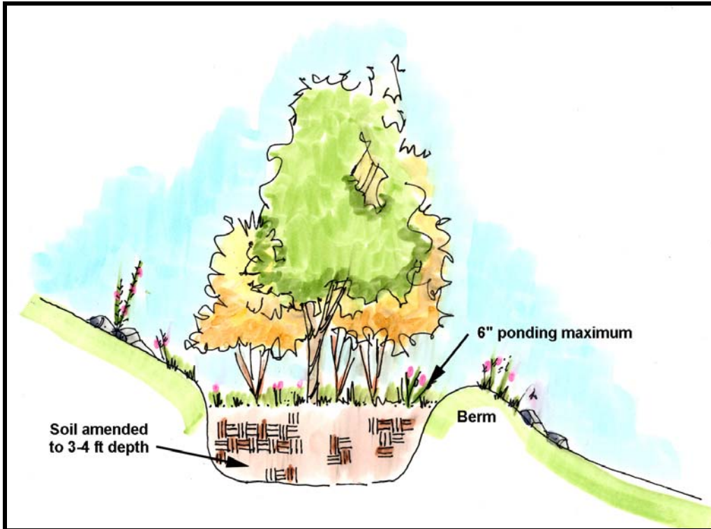
Figure 30. Tree cluster planted on side slope of a storm water pond (Graphic by Matt Arnns)
