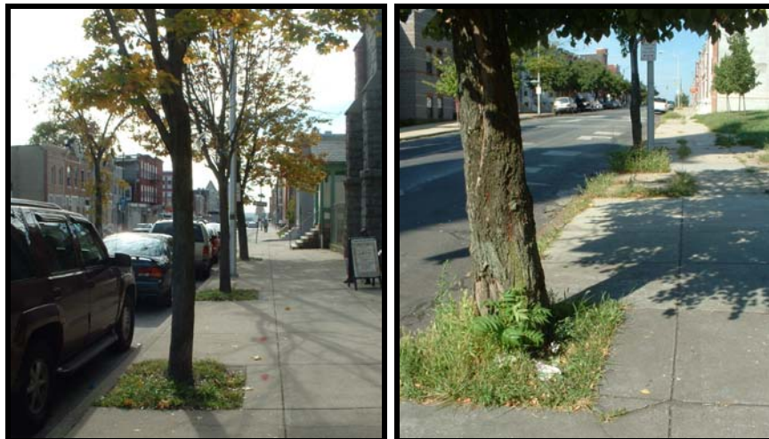
Figure 5. Typical urban tree pits only provide about 50 cubic feet of soil
