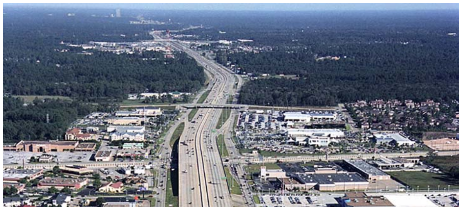
New development often eliminates almost all existing tree cover with little replacement planting. The elimination of trees and the addition of mostly impervious surfaces creates challenges for managing runoff while adding to the urban heat island effect.
