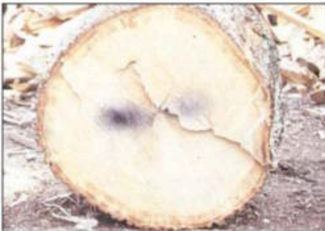
The discoloration on the end of this log indicates the presence of metal near the stained area.
