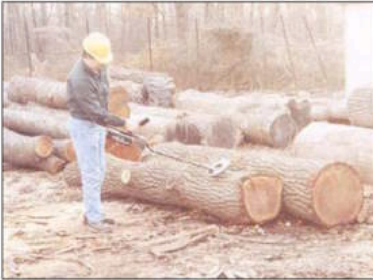
Following a thorough visual inspection of the sawlog, use a metal detector to carefully scan for metal hidden within the log.
