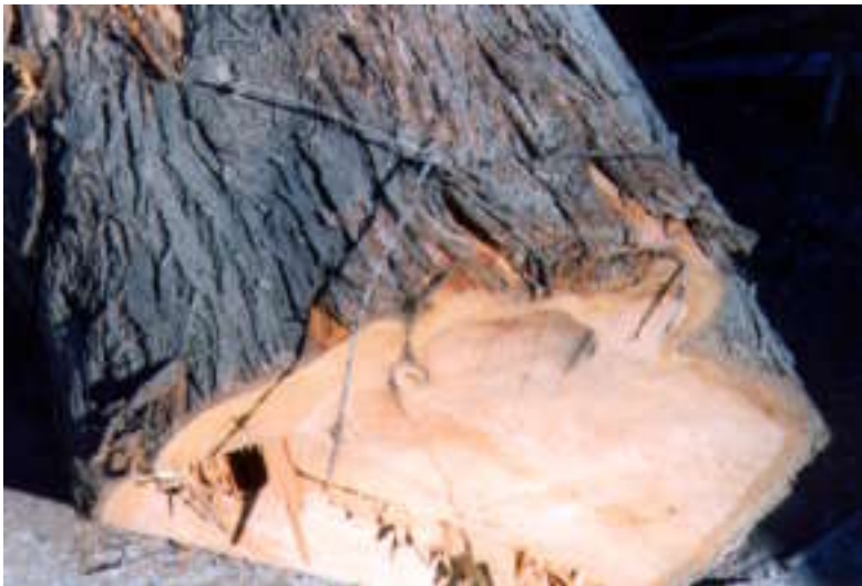
Figure 8.1. Wire is one of the more common embedded materials found in the trunks of trees removed from rural roadsides. In this example, the wire is easily detected. When an object is completely embedded, the only visible indicator may be a dark stain at the end of the log.
