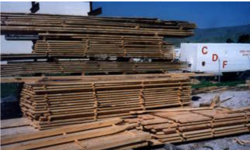
Figure 5.12. Both softwood lumber, shown here, and hardwood lumber produced by Pacific Coast Lumber were dried in the CDF portable, demonstration dry kiln. Equipped with an Eback T2000 dehumidification unit, it has the capacity of about 1,500 bd. ft. It takes about 30 to 60 days to dry softwood and hardwoods respectively.
