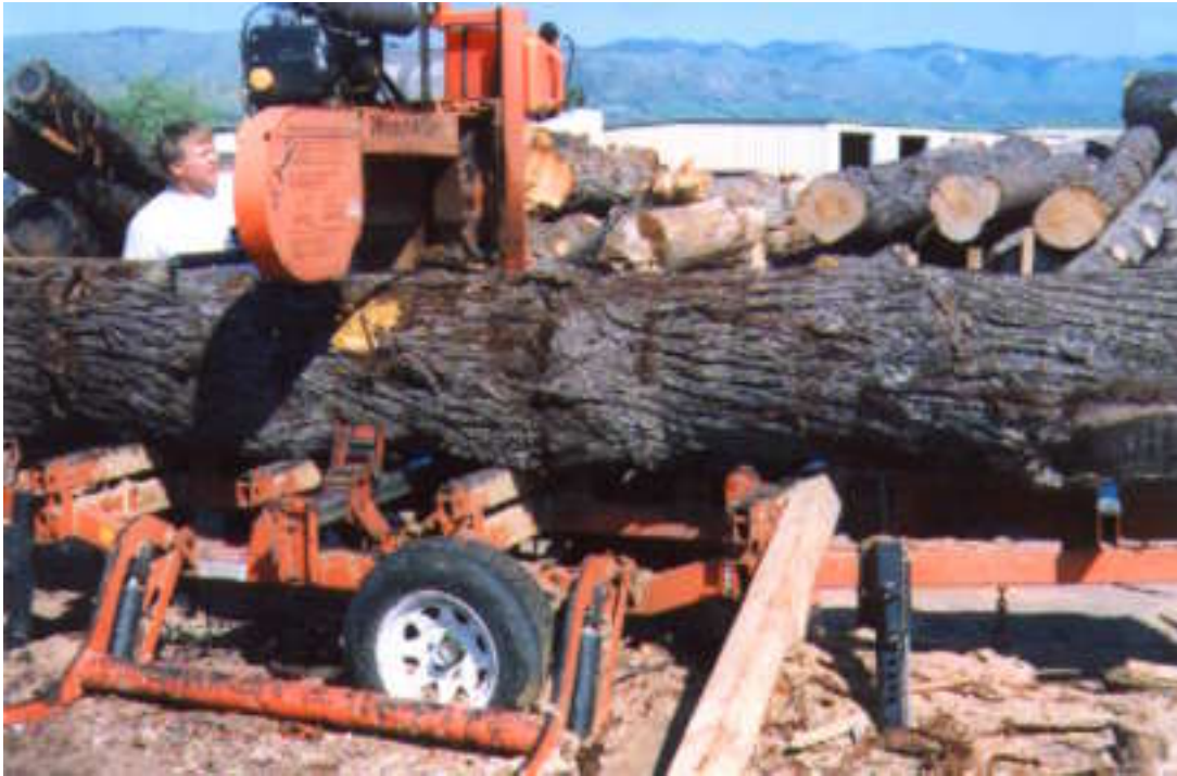
Figure 5.10. Don Seawater's Wood-Miser band mill is beginning the first cut into a 24-inch walnut log.
