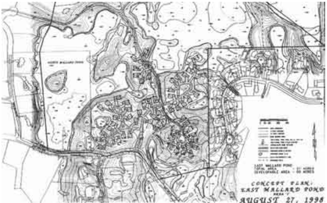
Figure 3-2. A comprehensive Landscape Resource Map of a subdivision such as this example from North Oaks, Minnesota shows location of wooded areas, individual trees, water bodies, proposed developable sites, and conservancy areas. Source: Minnesota DNR 2000.
