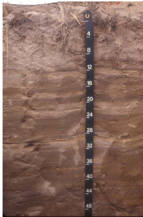
Figure 8.1b: Profile of a Big Apple soil, which formed in dredged spoil.
