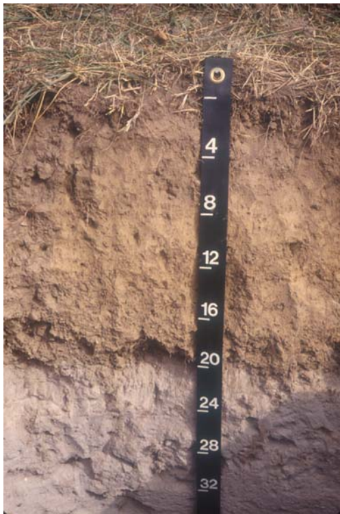
Figure 8.1a: Profile of a Verrazano soil, which formed in loamy fill over natural sand.
