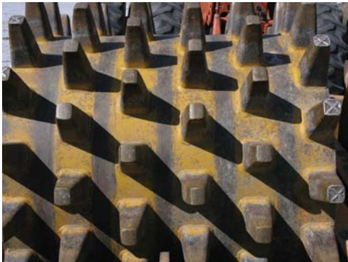
Figure 5.3: Sheepsfoot rollers compact soil.
