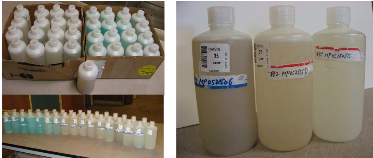
Figure 10: Water quality testing, water samples from each test were stored in a 500 ml water bottle for water quality analysis. The green-blue water color in the left image is the synthetic runoff that was mixed with natural runoff and fertilizer. The image in the right shows the runoff before (left) and after passing through the soil column (middle and right).
