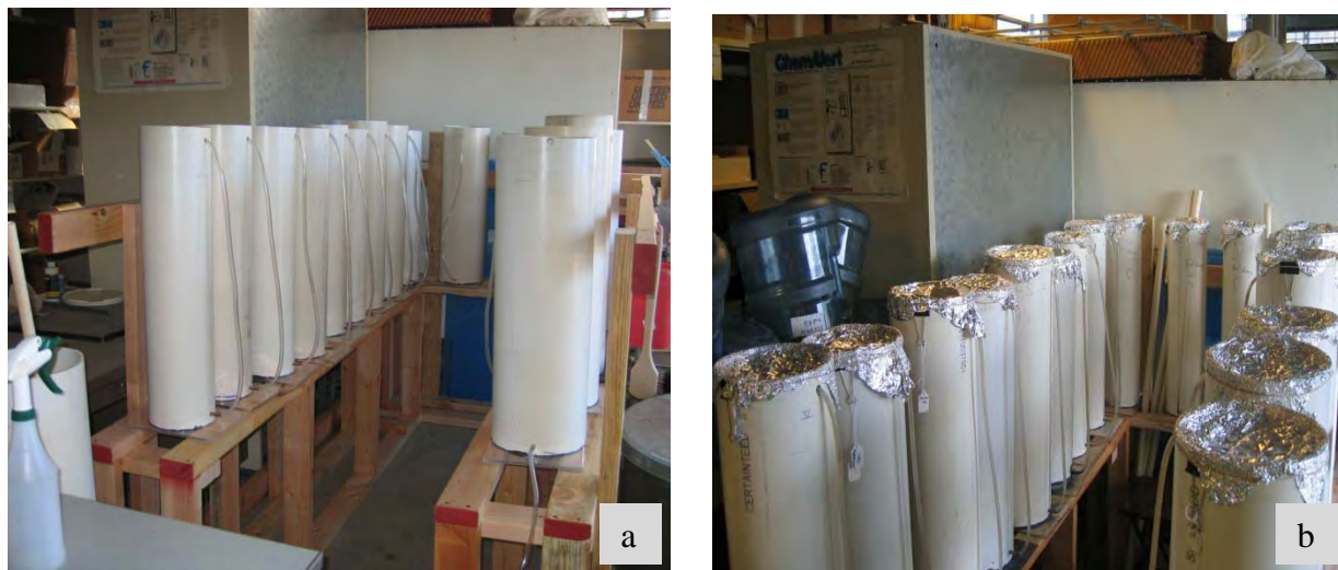
Figure 5: System setup (a) Columns were set on a wooden structure (b) The top of each column was wrapped with an Aluminum foil sheet to prevent contamination of the system and evaporation.
