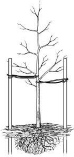
Figure 3. One example of how to properly stake a tree.
