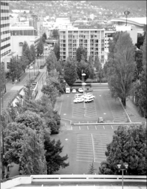
Perimeter plantings can screen views of the paved area, but may not provide much parking lot shading
