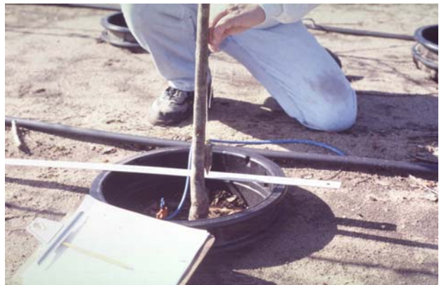
Fig. 6. Tree lean was measured using a plumb-bob and a centimeter gauged ruler.
