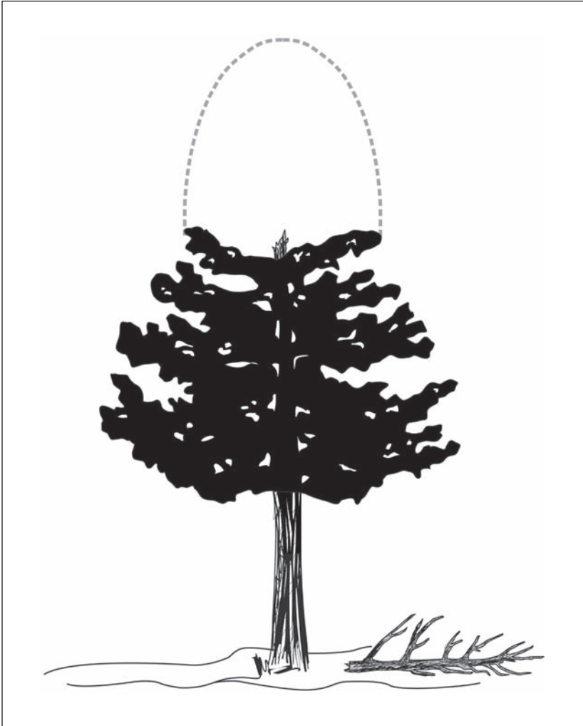
Figure 2.9—Missing portions of a tree crown are reconstructed to determine the crown density outline.
