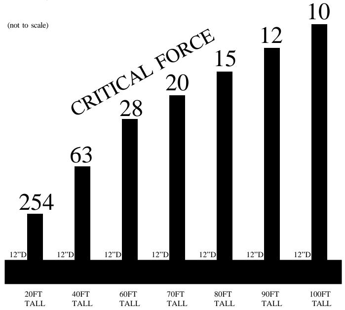
Figure 3: For each stem, with increasing heights and with diameters all equal to 12 inches, the relative critical forces required to propagate Euler buckling are listed.
