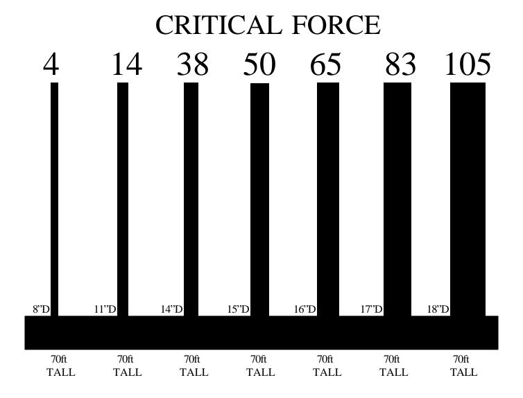
Figure 2: For each stem, with heights all equal to 70 feet and with increasing diameters, the relative critical forces required to propagate Euler buckling are listed.
