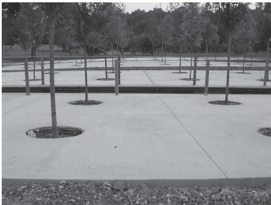
Figure 8 —Testing is being carried out at the Bartlett Tree Experts Laboratory in Charlotte to study different paving materials to reduce conflict between infrastructure and trees.
