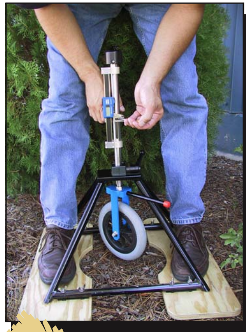
Figure 31—Using the rotational penetrometer to determine whether a surface is firm and stable.
