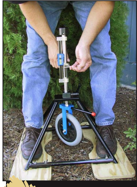
Figure 125—Using the rotational penetrometer to determine whether a surface is firm and stable.
