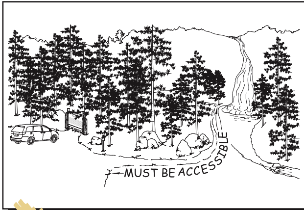
Figure 107—There are no uncorrectable barriers between the end of this trail and the waterfall, so this section of the trail must be accessible.
