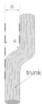
Fig. 12. The angle 'A' can be no more than 30°. The distance 'B' can be no more than the trunk diameter.
