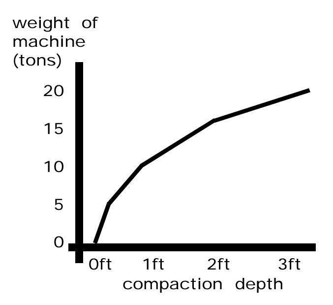
Figure 2: Depth of soil compaction under machines of various weights. (after Randrup 1999)
