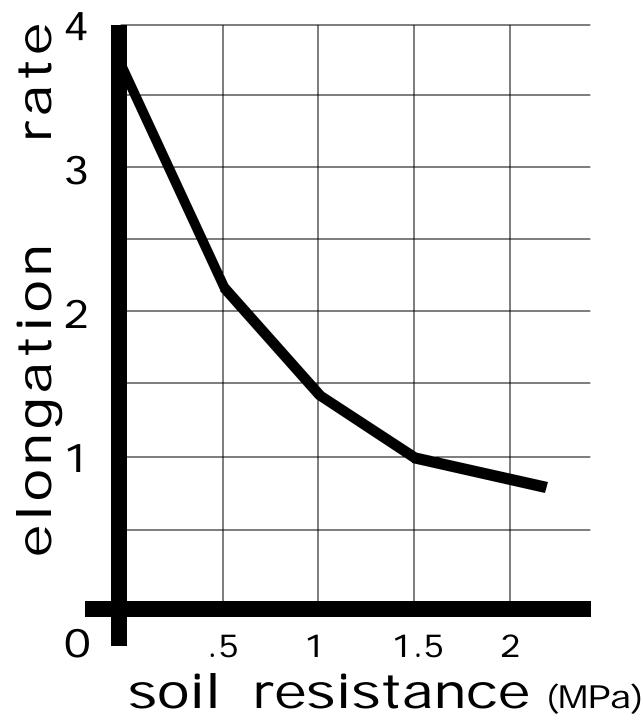
Figure 1: Soil penetration resistance and root elongation rate. (after Rendig & Taylor 1989) (1 MPa = 100 kPa • 1 bar)
