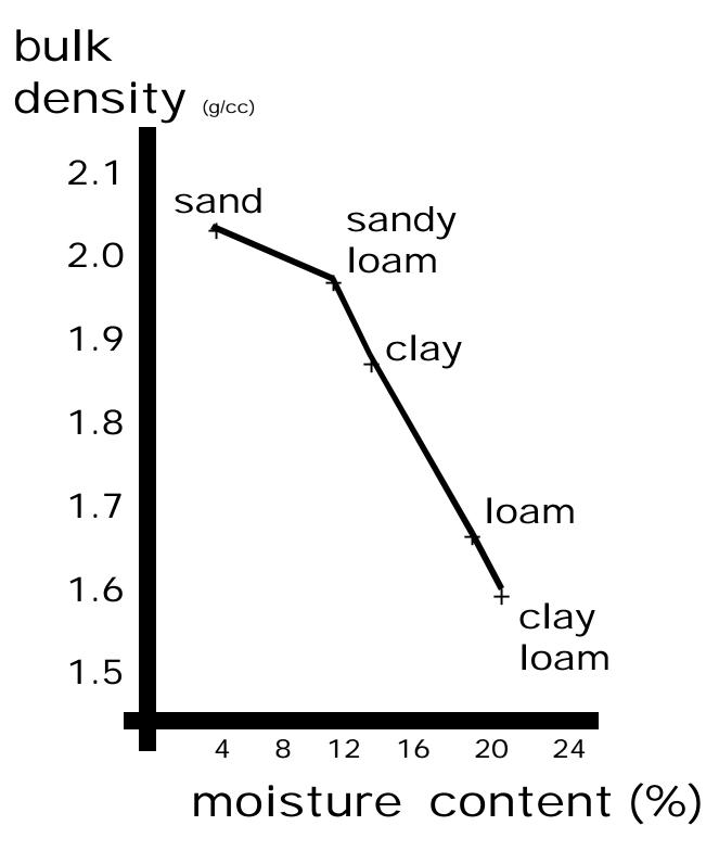
Figure 1: Maximum compaction capacity by moisture content. (after Craul 1994)
