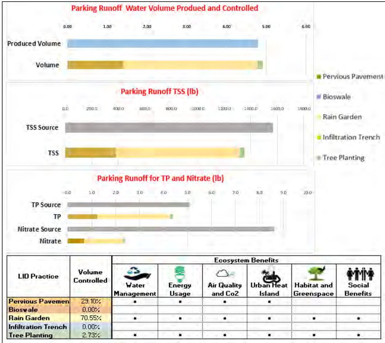
Figure A-10. Estimated pollutant load reductions and other ecosystem benefits from parking and road runoff for selected LID practices for the 2-year, 24-hour design storm.
