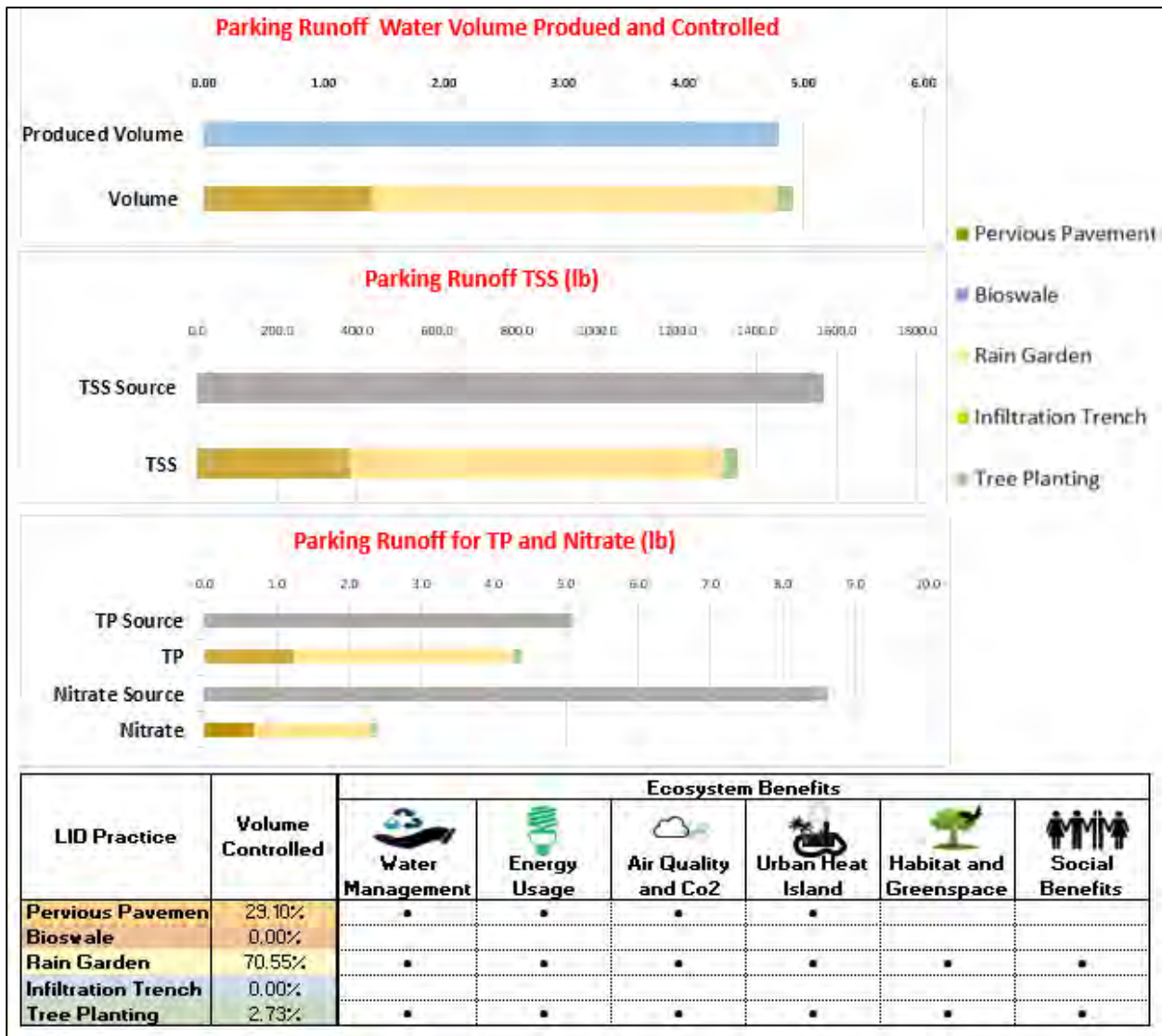
Figure 8.25. Estimated pollutant load reductions and other ecosystem benefits from parking and road runoff for selected LID practices for the 2-year, 24-hour design storm.
