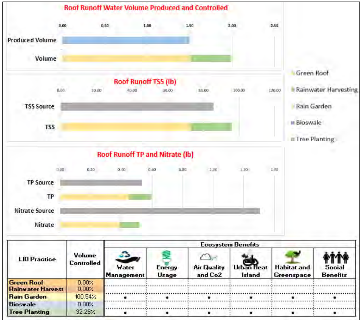
Figure 8.24. Estimated pollutant load reductions and other ecosystem benefits from roof runoff for selected LID practices for the 2-year, 24-hour design storm.
