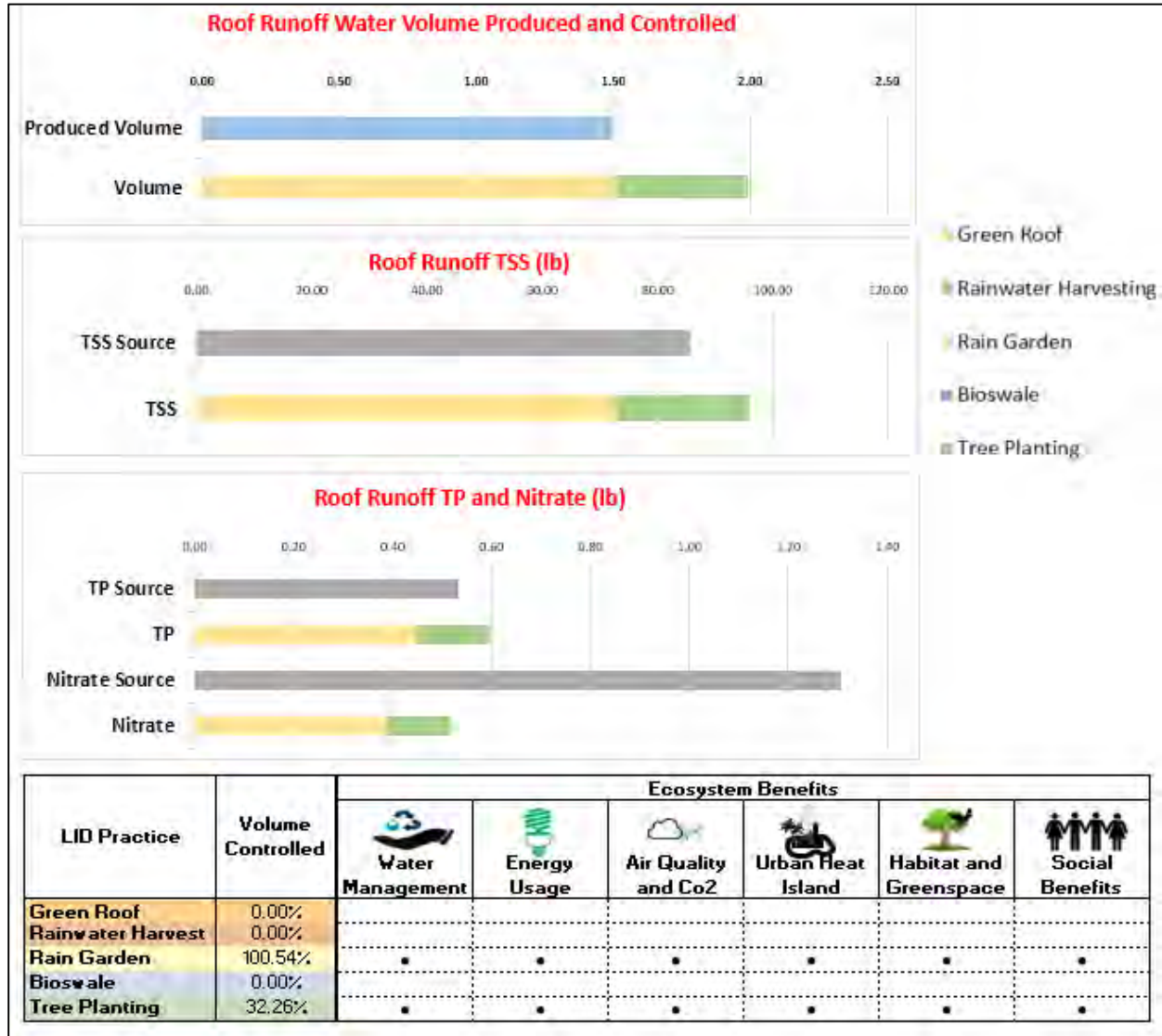
Figure A-9. Estimated pollutant load reductions and other ecosystem benefits from roof runoff for selected LID practices for the 2-year, 24-hour design storm.
