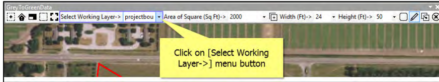
Figure 4.13. How to select the appropriate working layer on the G2G Data toolbar.
