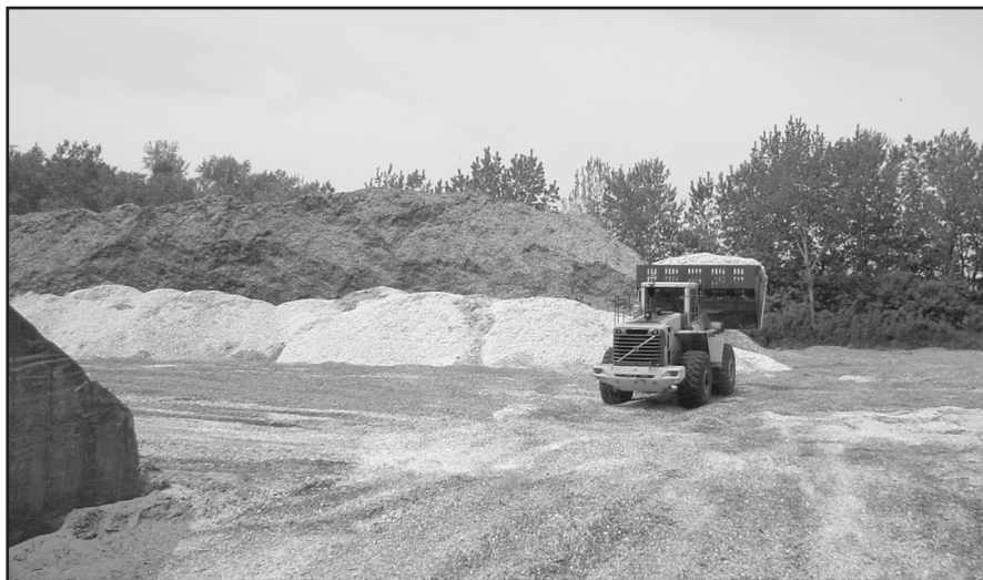
Figure 1. Wood chips are stored in long, low piles to prevent fermentation. PHOTO COURTESY OF McNEIL GENERATING STATION.
